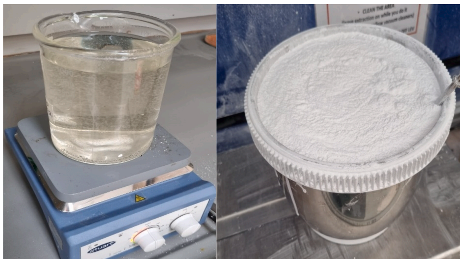
Fig. 3. Aluminum fumarate preparation for coating (a) distilled water mixed with binder (b) mixing distilled water and binder with adsorbent material powder.
