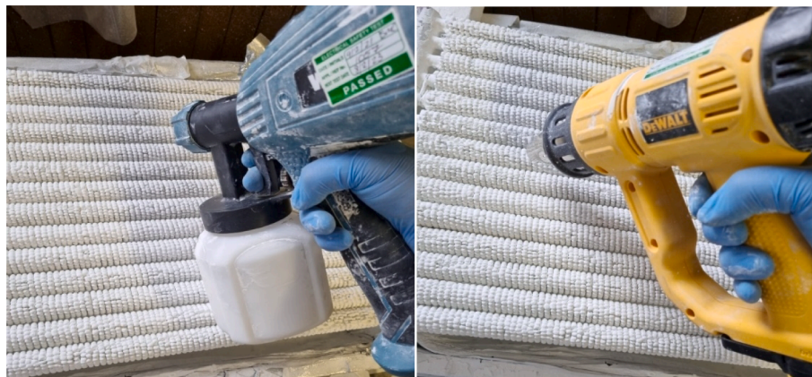
Fig. 5. (a) Adsorbent material spraying and (b) initial drying before placing the heat exchanger in the oven.
